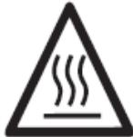
**Risk of burns!** Do not touch heating element pipes and nozzles used when hot. Let the device cool down. Do not point the hot air jet at persons or animals.
