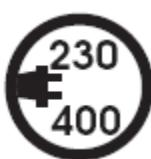
**The mains voltage** specified on the device's type plate must correspond to the mains voltage. Tools with a fix connection must be connected to a separator (e.g. mains switch). Special connecting conditions according to IEC/EN 61000-3-11;  $Z_{max} = 0,039\Omega + j 0,025\Omega$  for short time rating (30 minutes);  $Z_{max} = 0,026\Omega + j 0,016\Omega$  for continuous operation. Consult your local electricity board if necessary.
